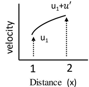
Velocity profile for turbulent flow
